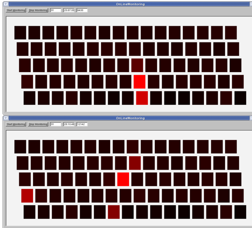
Figure 3.29: Examples of on line monitoring, color red intensity is proportional to QDC or TDC counts. On top we report detector response to a muon beam interacting on green dot of Figure 3.28, and on bottom the same but on blue dot: we can observe how in bottom figure there is an evident channel inversion.
