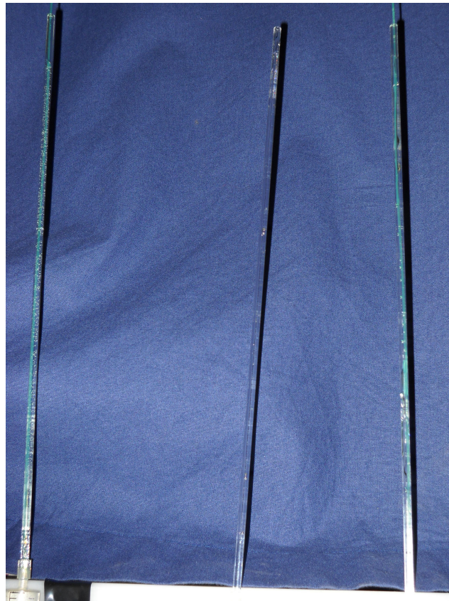
Figure 4.17: Here are reported the results of some tests did in order to chose the optical glue, to test different glues a glass capillary has been used in order to simulate the hole inside each bar, moreover a fiber has been inserted.
