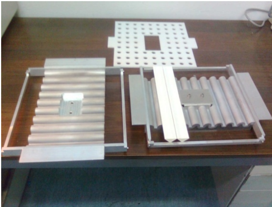
Figure 4.8: Jig used to align bars during gluing, on top Teflon mask to distribute glue spot.
