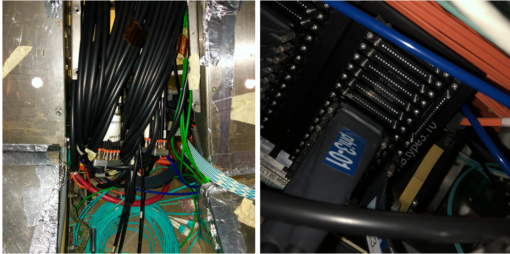
(a) Megatile fibers connected to RMs. (b) close-up of fiber-RM connection.
