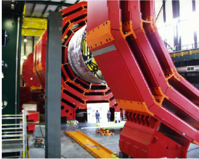
Figure 3.8: A photo of a yoke endcap disk, the central wheel with the vacuum tank, and an additional barrel wheel during magnet assembly in SX5.[44]
