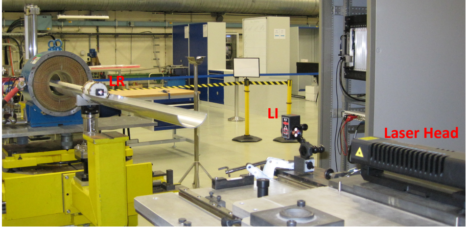
Figure 4.4: Laser head and linear interferometer (LI) and retroreflector (LR) for the position measurement.
