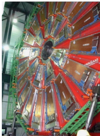
Figure 29: Cathode Strip Chambers mounted on a CMS Endcap [37].
