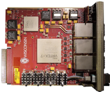
Figure 3.5: CTP7 [142] (left) and MP7 [143] (right) boards used in the upgraded CMS Level-1 Calorimeter Trigger.
