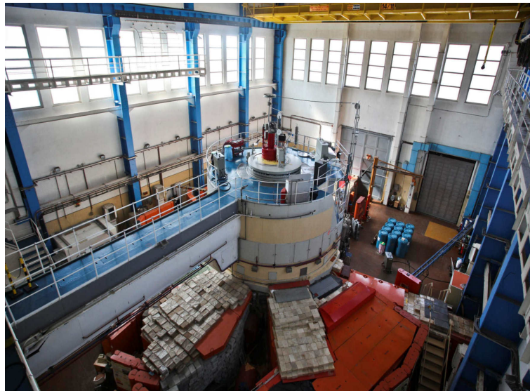
Figure 3.1: General view of the 10 MW Budapest Research Reactor Hall. The experimental beam lines exit the reactor on the left side and go across a thick shielding wall that separates the reactor hall and CNS Measuring Hall, where the PGAA and NIPS facilities are found.
