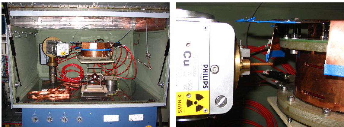
Figure 8.14: Left: Experimental setup for X-ray irradiation of the test chamber, showing the generator and the lifted detector; both inside a shielding box. Right: Collimator pointing to one of the field cage windows.
