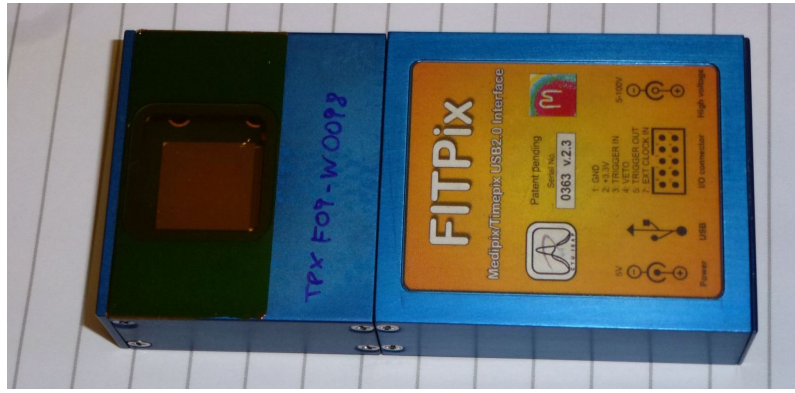
Figure 2.33: Timepix detector with a FITPix USB interface. The detector chip can be seen through a window on the left-hand side.
