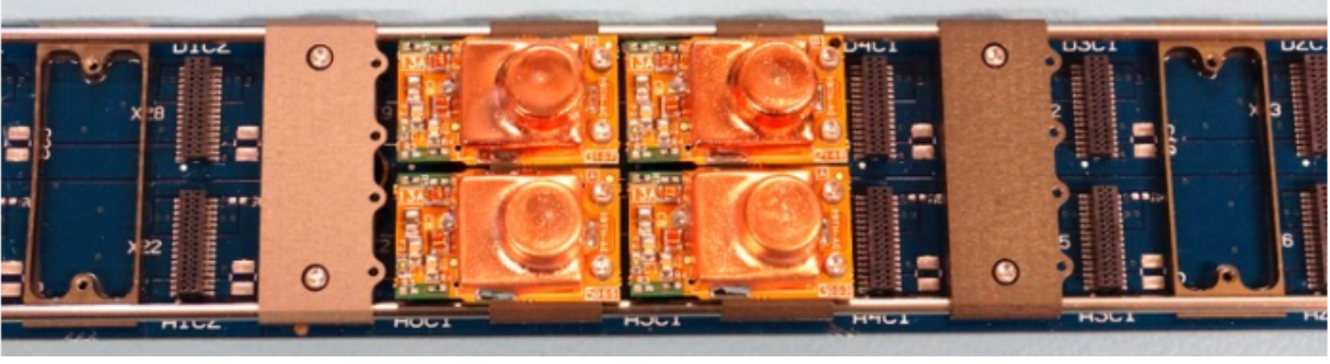
Figure C.2: Four DC-DC converters on the a bus board. A pair of the converters are analog while the other pair is digital [52].
