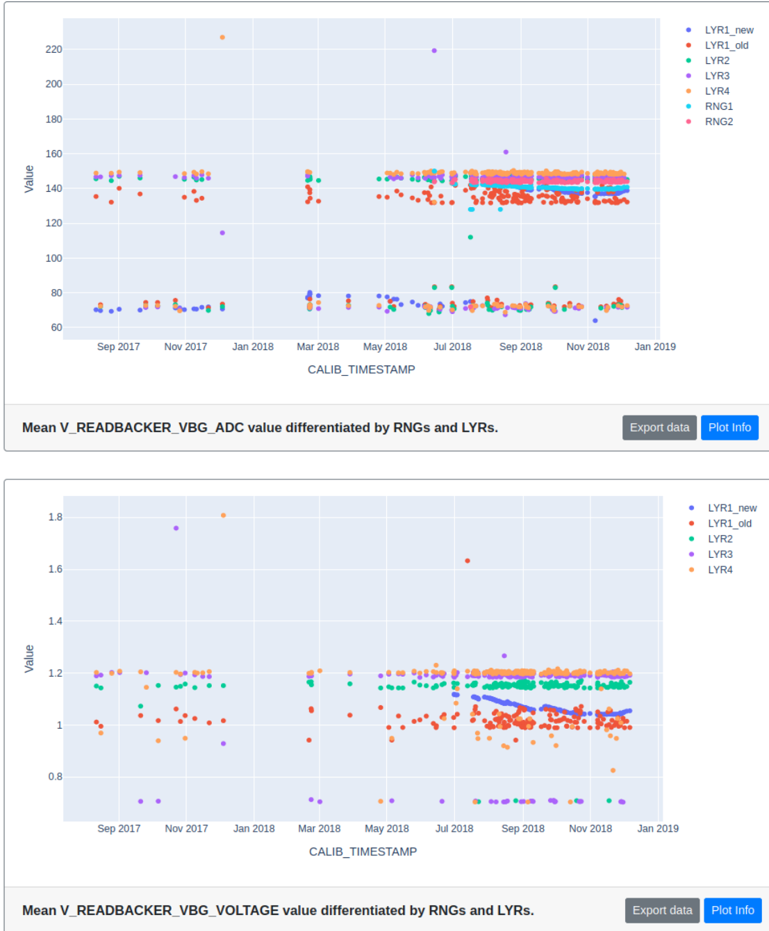
Figure 6.4: Average value of V_{bg} in ADC units (top) and after conversion to volts (bottom) for BPix layer 1 (old and new modules), layer 2, layer 3, layer 4, and FPix ring 1 and ring 2 during 2017 and 2018.
