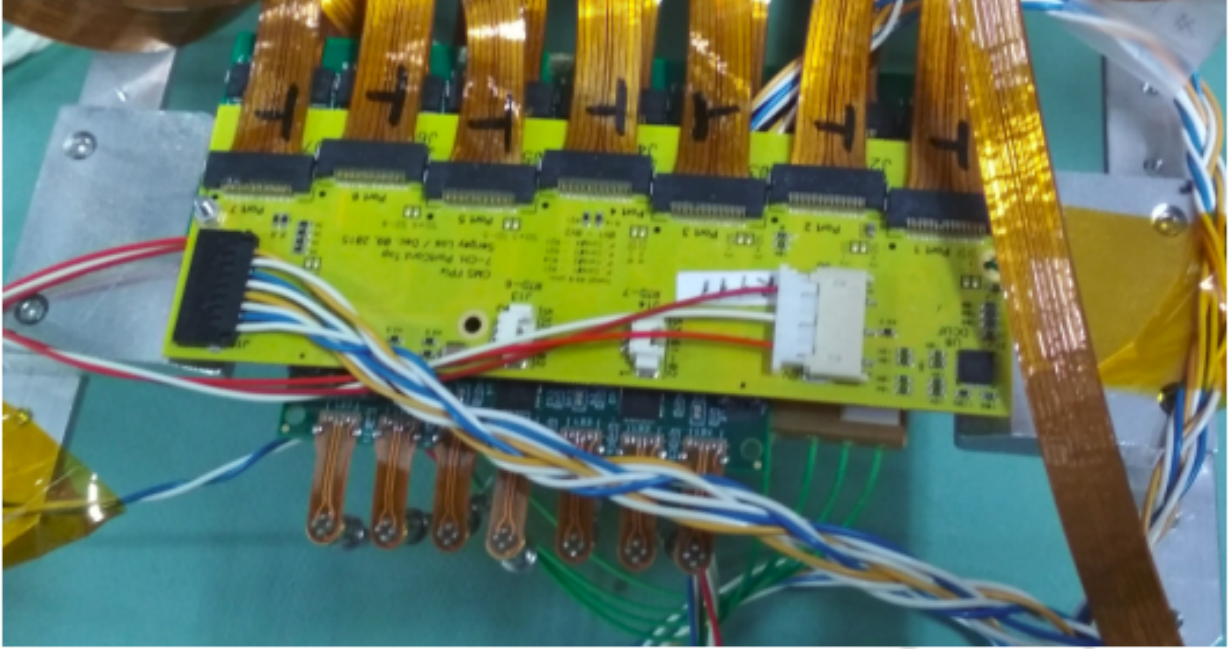
Figure C.3: Picture of a portcard used in an FPix test setup. [90].
