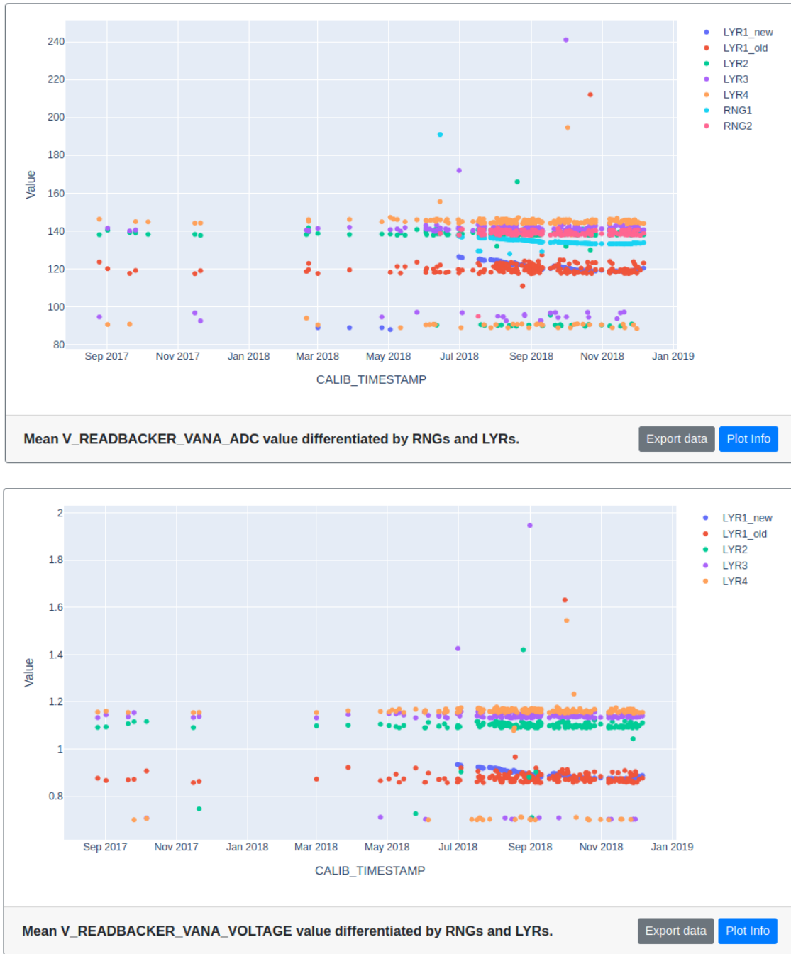
Figure 6.3: Average value of V_{\text{ana}} in ADC units (top) and after conversion to volts (bottom) for BPix layer 1 (old and new modules), layer 2, layer 3, layer 4, and FPix ring 1 and ring 2 during 2017 and 2018.
