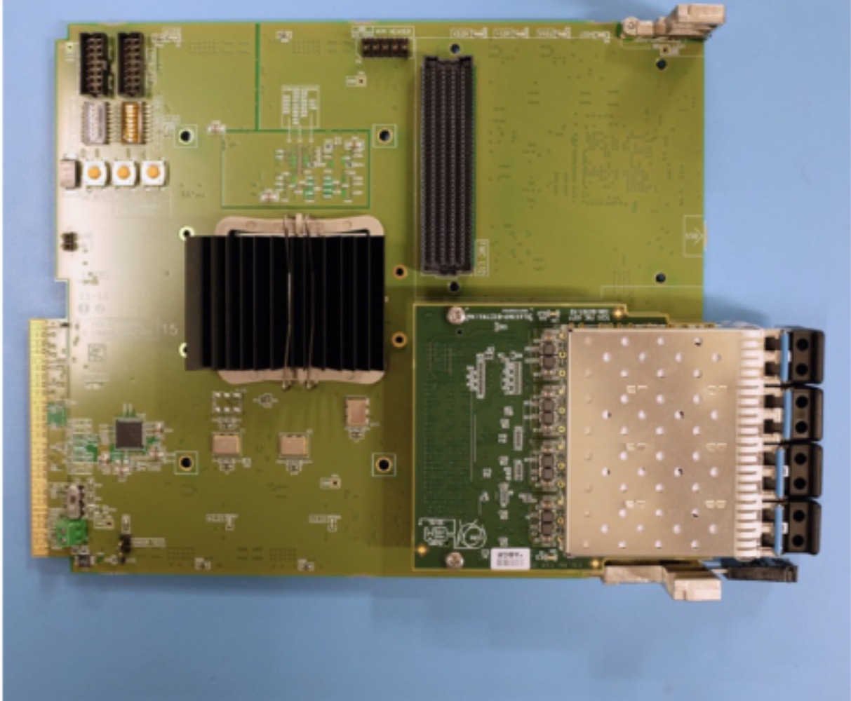
Figure 5.12: FEC (Pix and TK) cards have the same FC7 board as the FEDs but a different mezzanine card. TkFEC and PixFEC have the same hardware and differs only in firmware. BPix uses 80 FEDs, 8 PxFECs and 2 TkFECs. FPix uses 28 FEDs, 8 PxFECs and 1 TkFEC [59].
