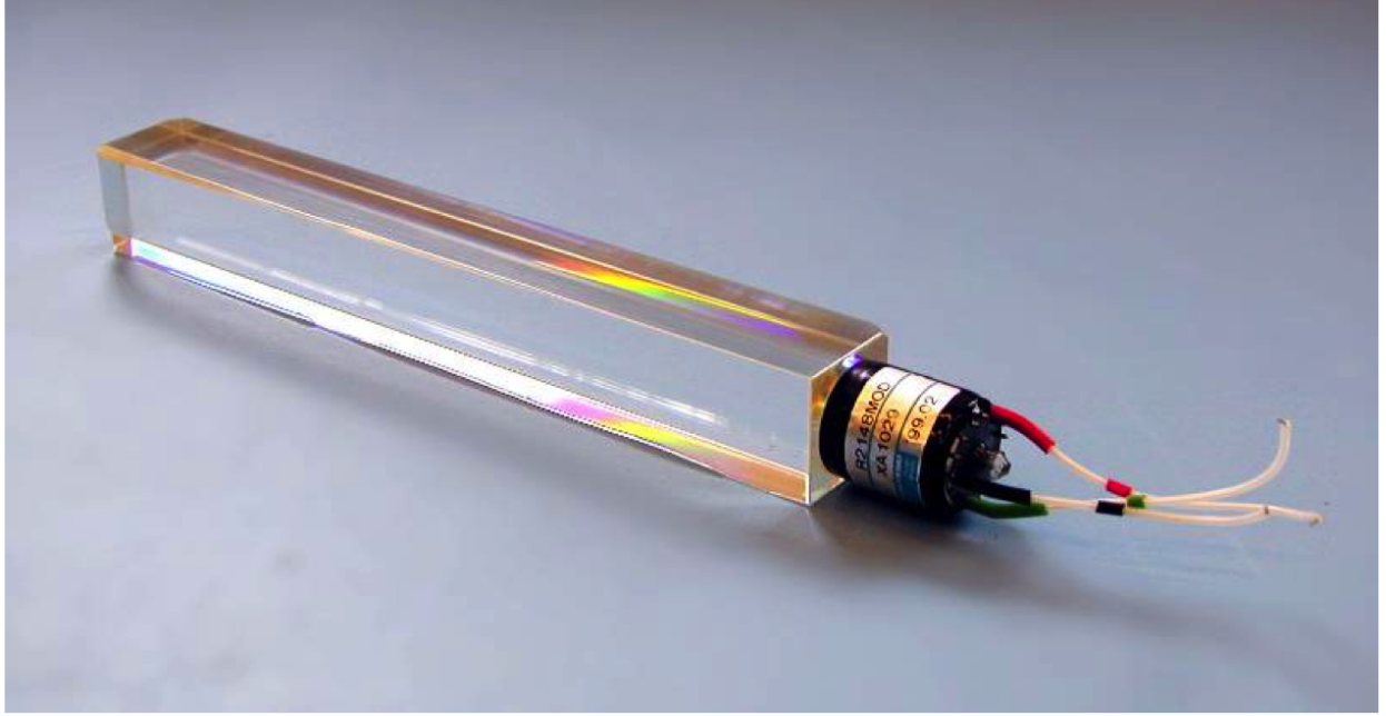
Figure 4.2: ECAL crystal with the photo-detector [40].
