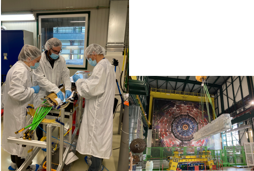
Figure 5.16: Part of FPix detector undergoing cooling repairs (left) and a part of BPix being craned over from the clean room to the CMS underground tunnel prior to installation (right).
