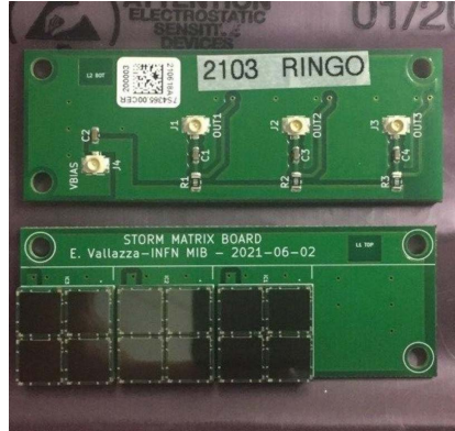
Figure 3.3: The photodetection system, consisting of three SiPM matrices connected on a readout board. V_{bias} (the J4 connector) is the common bias for the three matrices.
