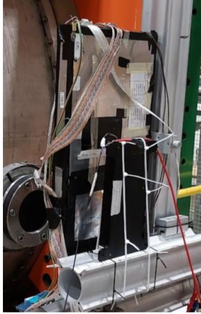
Figure 3.19: The trigger scintillator mounted downstream of the second beam chamber in the setup on the H2 beamline.
