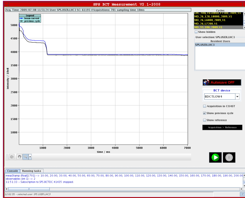
Figure 4.28: An example of beam current behavior during the SPS experiments observed from the monitor of the Beam Current Transformer: the losses corresponds to the injection an acceleration phase, on the flat-top there is not significant loss on this scale and the beam lifetime is good. The two curves represent two consecutive turns: we can infer that the reproducibility of the machine, in that condition, was good.
