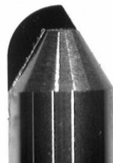
Figure 3.13. On the left single crystal diamond controlled waviness tool, on the right CVD ball end mill (Technodiamant 2011).
