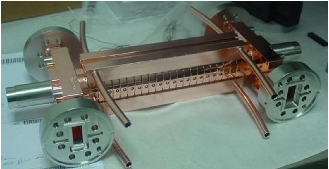
Figure 1.1. CLIC accelerating structure prototype (Picture courtesy of CERN).
