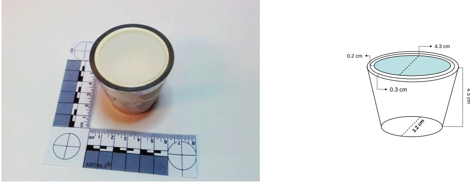
Figure 2.2: On the left a picture of the truncated cone \text{LaBr}_3(\text{Ce}) crystal used in the IS474 experiment. On the right a scheme of this same crystal with its dimensions and that of its encapsulation.
