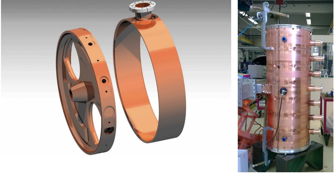
Figure 1.16: Left: Discs and rings before welding. Right: CERN's Linac4 hot prototype of PIMS
