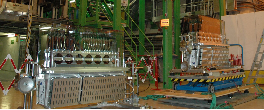
Figure 3.21: VELO2 being transported from the underground cavern to the exhibition area at UX85. The outer perspex casing has been removed during transport.
