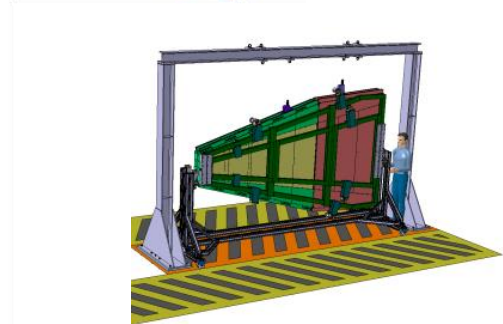
Figure 3 Tooling for assembly of the sectors [5]
