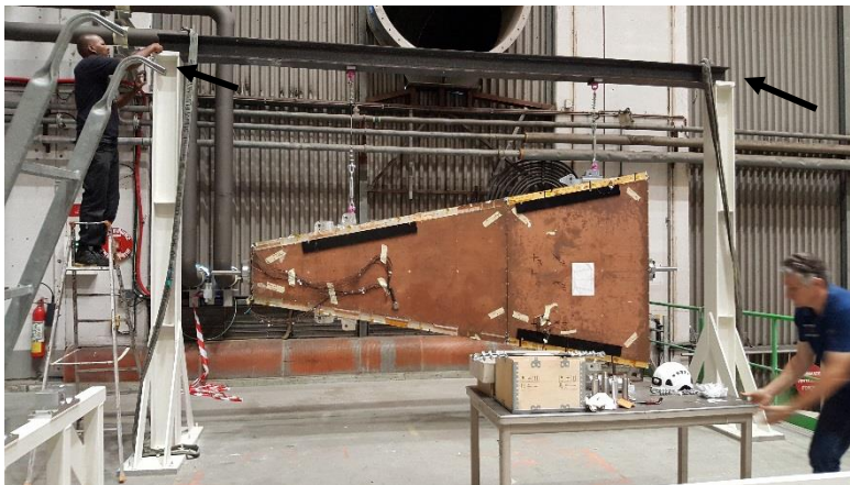
Figure 25 positioning the lifting bar to the assembly station with screws
