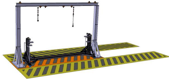
Figure 11 assembly frame with trolley [16]
