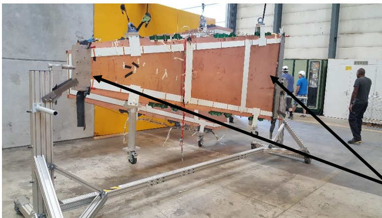
Figure 20 Place sTGC into the trolley with the Christmas tree.
