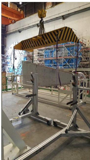
Figure 18 Transport basket hanging in lifting tool
