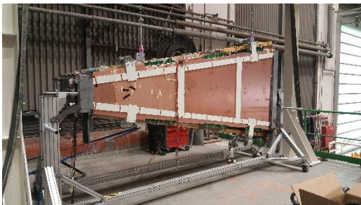
Figure 36 Positioning of the sTGC in front of the MM-DW
