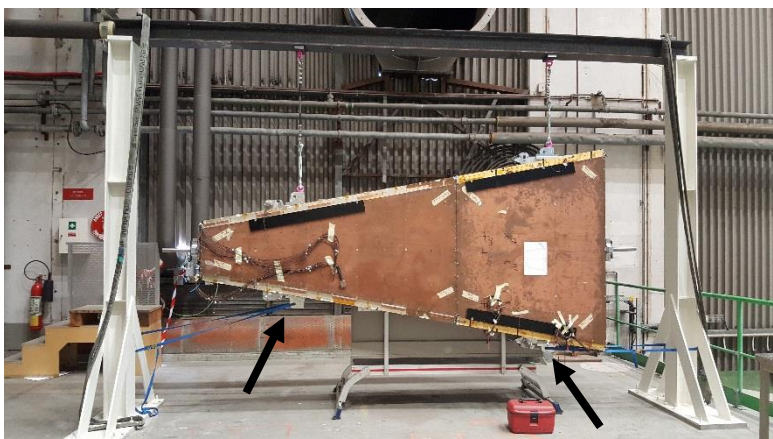
Figure 24 Here the pillar must be installed and connected to the grabber mounts
