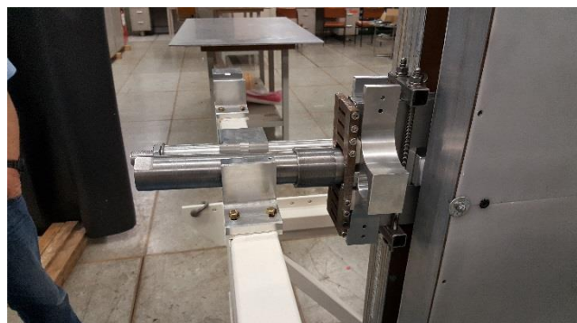
Figure 13 Connection of the cross into the transport basket with fixing bar
