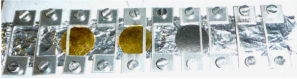
Fig. 4.11: The photograph of gold and platinum foils fastened in the SSP sample holder. It was possible to place up to 10 foils into the holder, however, only three foils were irradiated. The holder geometry was fixed and the ion beam was steered in order to irradiate the individual foils.
