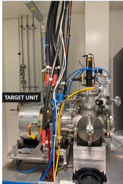
Fig. 3. Set-up for Sc thermal release experiments.
