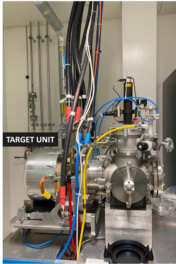
Figure 2.10: Set-up for Sc thermal release experiments
