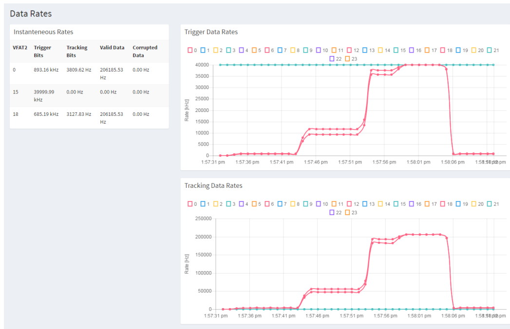
Figure 6.23 – Screenshot of the page of the web application used to monitor the hit rates.
