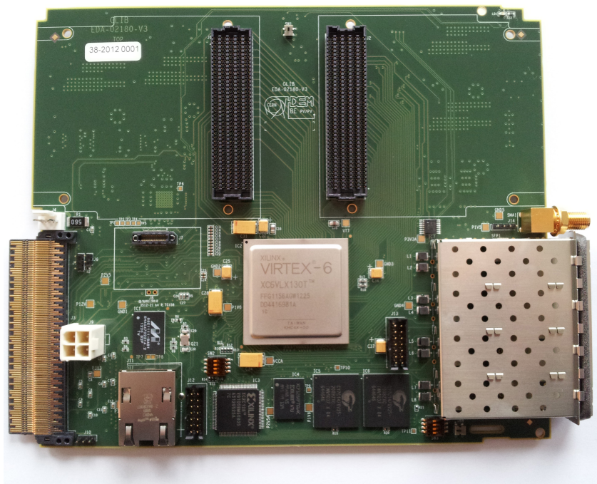
Figure 5.16 – Picture of the GLIB AMC equipped with a Xilinx Virtex-6 FPGA, four SFP optical cages, and two extension headers that can accommodate custom electronics and are used as back-end electronics [37].
