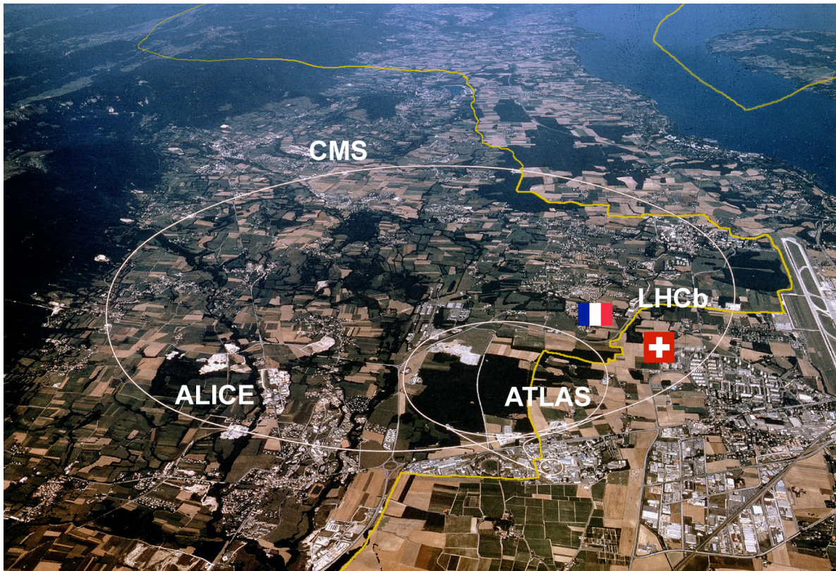
Figure 2-1. An aerial view of the LHC landscape. The French-Swiss border is indicated by the yellow line and the LHC tunnels are outlined in white. The triangular building complex just below ATLAS in the picture is the main campus of CERN. Picture taken from Ref. [3].
