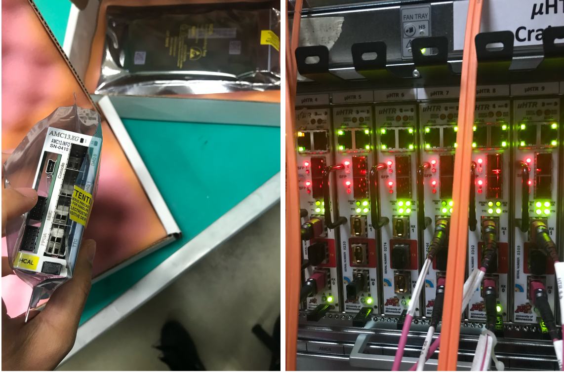
Figure 3.15: On the left is a new AMC13 tested at 904 with the \mu HTRs in a selected Back-End Crate shown on the right.
