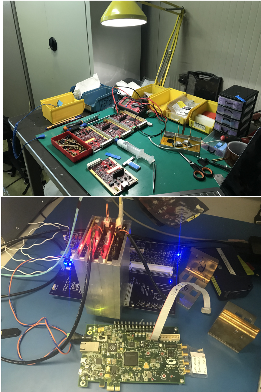
Figure 3.16: The top picture shows an ngCCM being reworked to add heat sinks to mitigate the VTRx RSSI drift issue which was related to the communications loss in the HCAL endcap. The right shows a reworked ngCCM being tested on a spare backplane.
