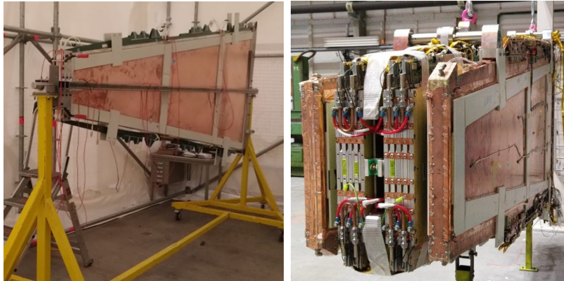
(b) Left: A sTGC wedge. The white frame outlines the individual quadruplet modules that have been glued together into a wedge. Right: A completed sector, with two sTGC wedges on the outside and two micromegas wedges on the inside.
