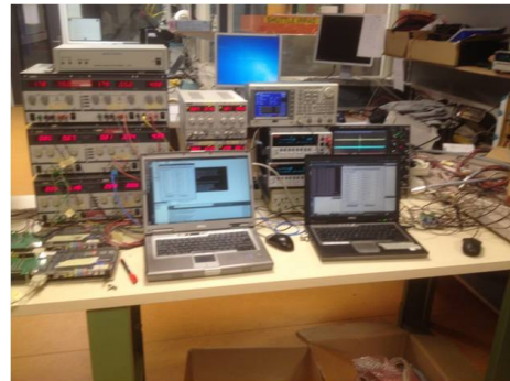
(a) Samples mounted on the irradiation table (b) AMS V4 test setup in control room
