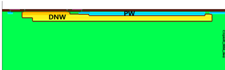
Figure 4.56 – Cut-plane of versionB doping
