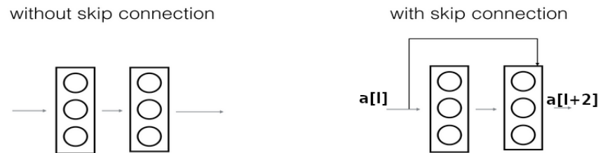
Figure 2.12: A ResNet block showing a “skip-connection”
