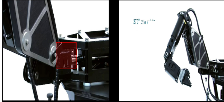
Figure C.16: Some failed detections from inference of the DetectNet model, a FP ( left ) and a FN ( right )
