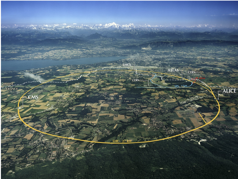
Figure 3.1: Illustration of the layout of the Large Hadron Collider [62]. It has 26.7 km long circumference and crosses the border between France and Switzerland. It is buried 100 m below the surface (on average). The LHC provides data to four main experiments, ALICE, ATLAS, CMS and LHCb.
