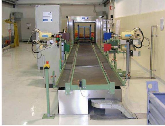
Figure 3.3: Photograph of the release measurement system (NUKEM) for packed waste at the research centre Ispra.
