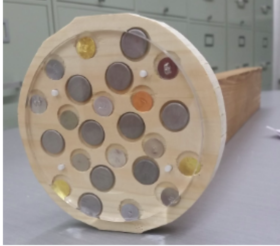
Figure A.3.1: An image of the foil holder used to put foils into the 6" beamport. The foils were placed in small holes bowed into a milled wooden disc and secured using a polyethylene disc attached to the face of the wood.
