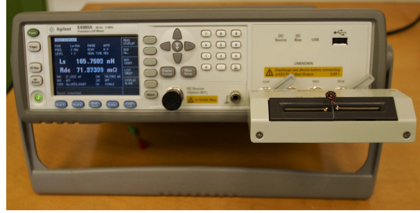
Figure 4.8: Picture of the LCR meter that is used for coil characterisation. A coil is attached to the test fixture.
