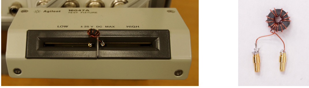
Figure 4.9: Picture of the LCR meter test fixture with an attached coil (left). On the right, a custom made toroid. Gold plated contacts have been soldered to the ends.
