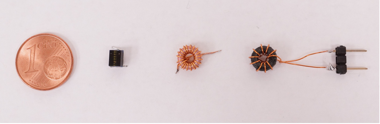
Figure 4.6: Picture of three different kinds of main inductors. On the left a 100 nH solenoid used as the default option on the bPOL2V5 evaluation board (Section 4.3). In the middle, a 220 nH toroid, which is used on the 2S service hybrid prototypes. On the right, a 100 nH custom made toroid. On the far left a 1 Euro Cent coil is given for scale.
