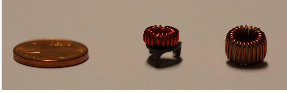
Figure 4.1: Main inductors of the 2S service hybrid DC-DC converter (middle) and the Phase-1 pixel DC-DC modules (right). Left, a 1 Euro Cent coin for scale [8].
