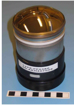
Figure 1.4.2: Hybrid photon detector [18].
