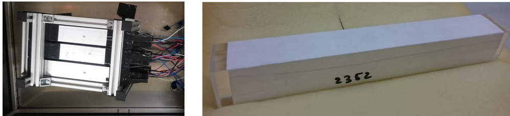
FIGURE 2.24. ( left ) STEFI on its mechanical support installed in the aluminum box. ( right ) A CMS endcap calorimeter crystal.
