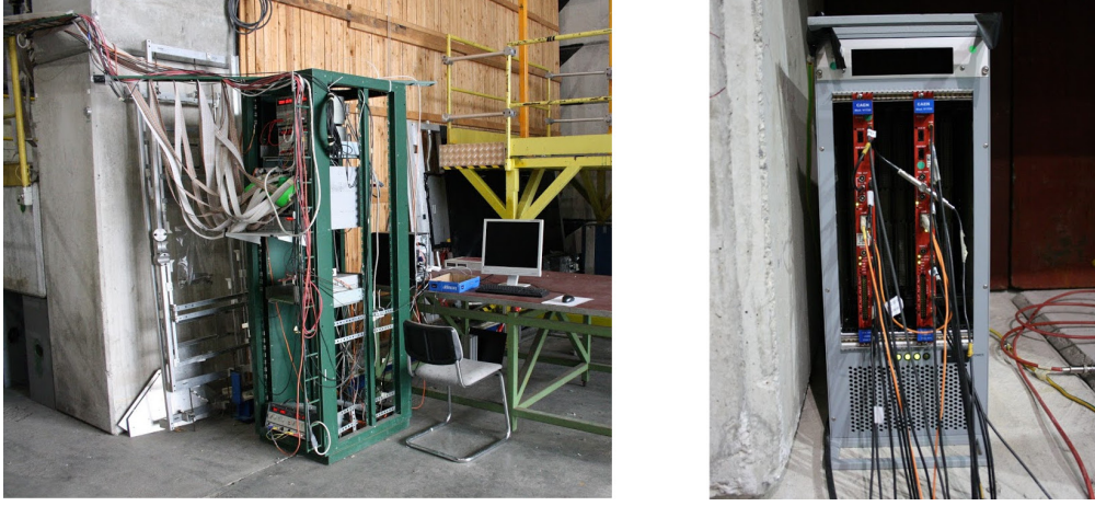
FIGURE 2.30. ( left ) VME crate with the VRBs, the trigger board and the SBS Bit3 620 board, the power supplies, the DAQ PC. ( right ) VME crate with the digitizers.
