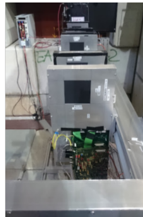
FIGURE 2.14. Tracking planes reference system; the beam enters the page; the x axis points towards Northwest.
