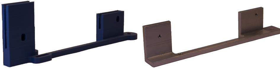
Figure 4.3.: On the left the 3D printed 8CBC2 right angle bracket is shown. The right picture shows the aluminum version, which was later used to improve grounding connections and reduce noise.
