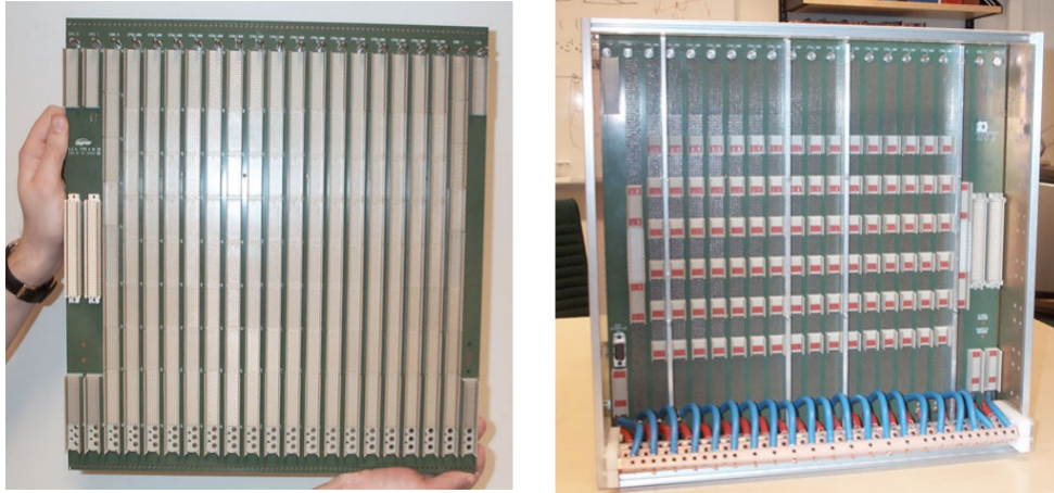
Figure 3.11: The Processor Backplane - front view where the modules plug in inside crate (left) and the back where cables plug in (right) [34]
