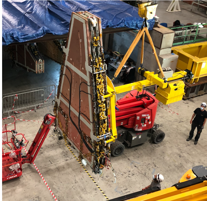
Figure 3.12: A large sector (C13) being lifted by a ceiling crane with a special turning tool in order to be installed onto the wheel. Other assembled sectors can be seen in the background, under the blue tarp covering.
