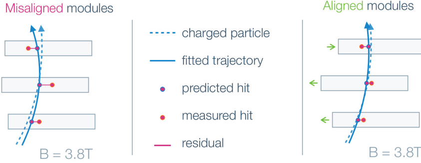
Figure 4.1: Sketch of a comparison between a fitted trajectory (solid blue) with misaligned (left) and aligned modules (right) [106]. The true trajectory of the charged particle is shown as a dashed blue line, while the predicted and measured hits are shown as blue-red and orange-red dots, respectively. The residuals between both hit types are visualized as solid red lines.
