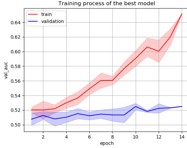
Figure 5.40: Evolution of AUC during the training of DNN to separate the nominal and systematic samples, using the same input features as the binary RNN.
