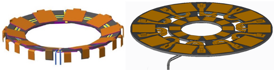
Figure 3.7: Ring layouts in the “Inclined Inner” (left) and “Inner Alternative” (right) proposals. Modules are depicted as orange rectangles [84].
