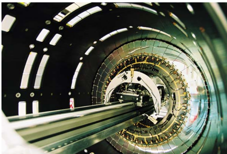
Figure 5.10: A disc held by the trolley on the supporting rails being inserted into its position within the cylinder support.
