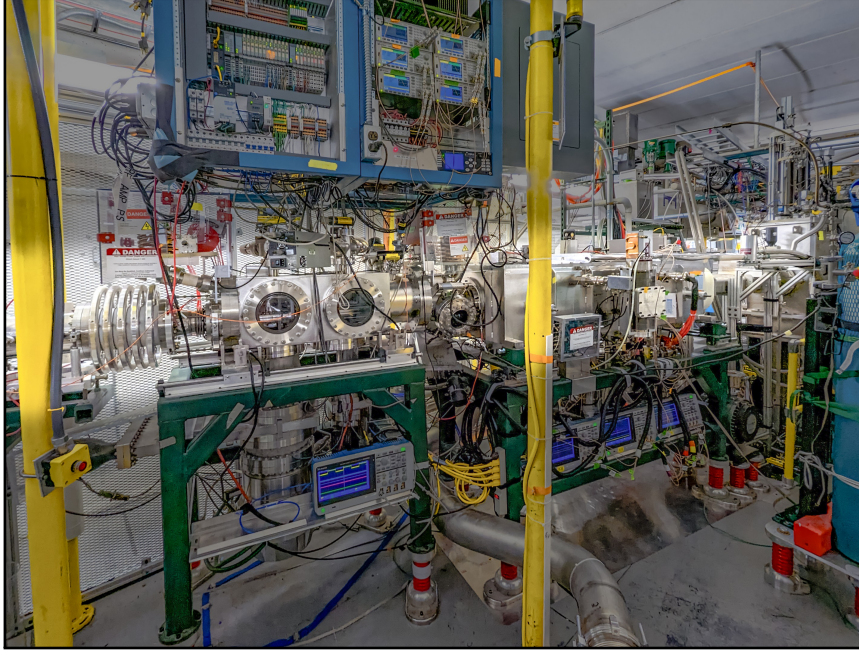
Figure 5.5: Advanced Gryogenic Gas Stopper (ACGS) at FRIB. The beam enters the gas cell at the right side of the photo and exits through the acceleration column on the left. Photo courtesy of Chandana Sumithrarachchi.
