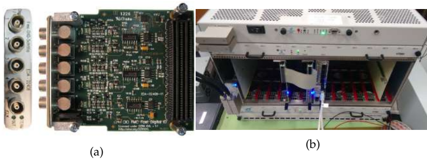
FIGURE 6.9: LEFT: The DIO5 FMC, very useful for its LEMO connectors which can be used to interface easily with the FPGA logic. RIGHT: Two interconnected FC7s, one running the emulator firmware and the other the DAQ firmware, to test the first features of the \mu DTC firmware. The FC7s are operated in a \mu TCA crate which can host up to 12 AMC cards. Centrally in the crate two half-width AMCs are visible: the MCH receiving the Ethernet cable at the bottom and the AMC13 at the top. The power modules for the crate are located at the far left of the crate.
