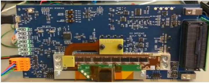
FIGURE 9.15: A 2S FEH carrying 8 CBC3.1 chips to which a CIC mezzanine card is connected to mimic a final 2S front-end hybrid. The CIC1 output data is routed back to the front-end hybrid and goes out of the hybrid over the connector which in a module would connect to the service hybrid, but here connects to a dedicated interface card.
