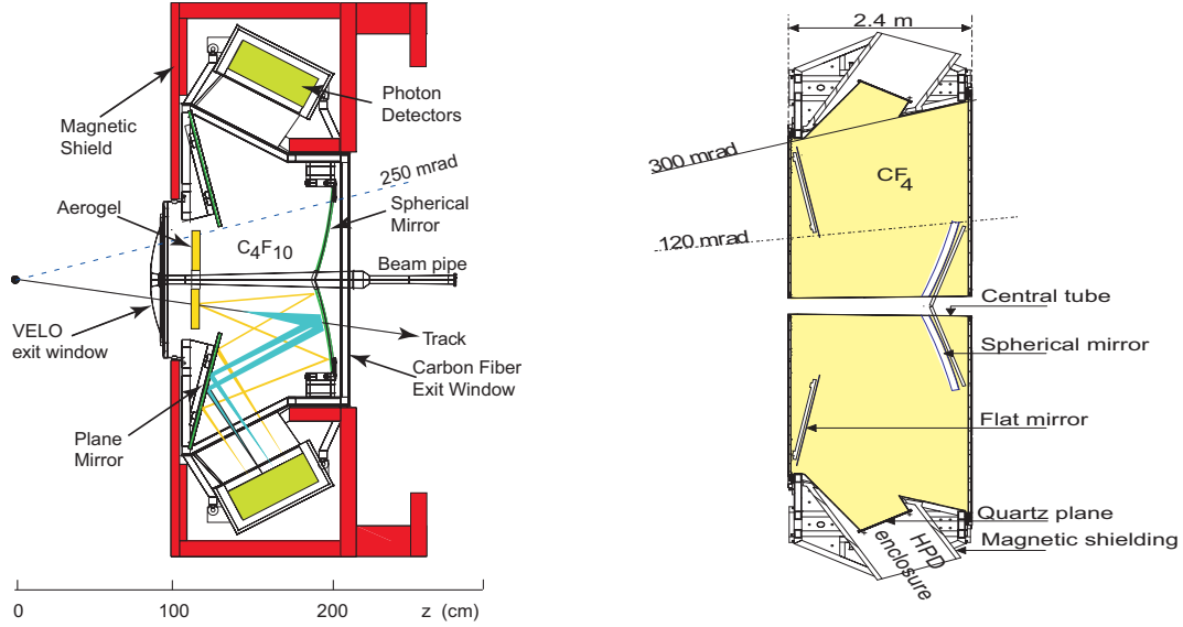
Figure 2.14: Left: RICH1 ( y, z ) plane sketch view. Right: RICH2 detector.
