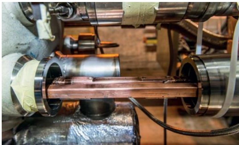
Figure 2-11: The bus bar in the LHC: Superconductors embedded in copper [46]
