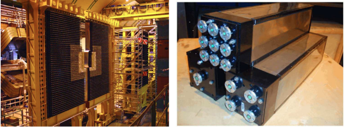
Figure 2.17: The electromagnetic calorimeter. The image on the left clearly shows the three different sections and the image on the right shows the three different types of modules [52].
