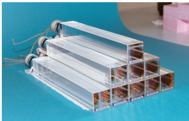
Figure 4.7: CMS ECAL Lead Tungstate Crystals ( PbWO_4 ).
