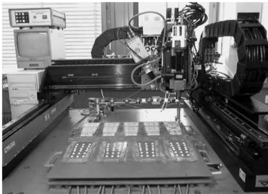
Figure 5.9: Automatic assembly robot as used in the CMS gantry centre in Bari, Italy. In front the assembly plate for four TID modules is visible. Behind it the supply platform and the tooling rack can be seen [Surrey 2001]
