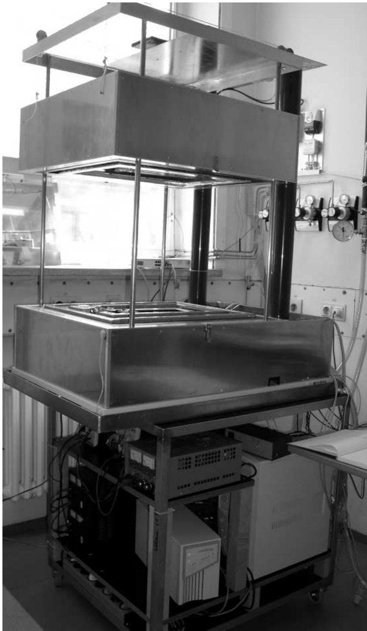
Figure 6.16: View on the Karlsruhe Fast Test Station (FTS). The cover can be lifted on rails. The counterweights for the cover run inside the pipes, which can be seen in the pictures background. Furthermore, the onion-like structure of the thermal insulation layer surrounding the small inner test volume is visible. On top (partly visible) and below the test station scintillators with photomultipliers are assembled, which can be used for system calibration and SNR measurements with cosmic rays. The electronics (motherboard and its hosted cards) are place behind the stations body and below the station (PC, power supplies, power pack and NIM logics). For ESD protection several GND connection points are available for the operator (e.g. cable visible at the lower front corner)
