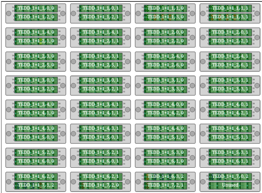
Figure 1.1. | Visualization of the optical tPP1 for sector tests, showing the MPO-to-LC adapter cassettes. The labels indicate which optical sectors correspond to which cassettes, for an exemplary sector test of a TEDD1+ odd top dee.
