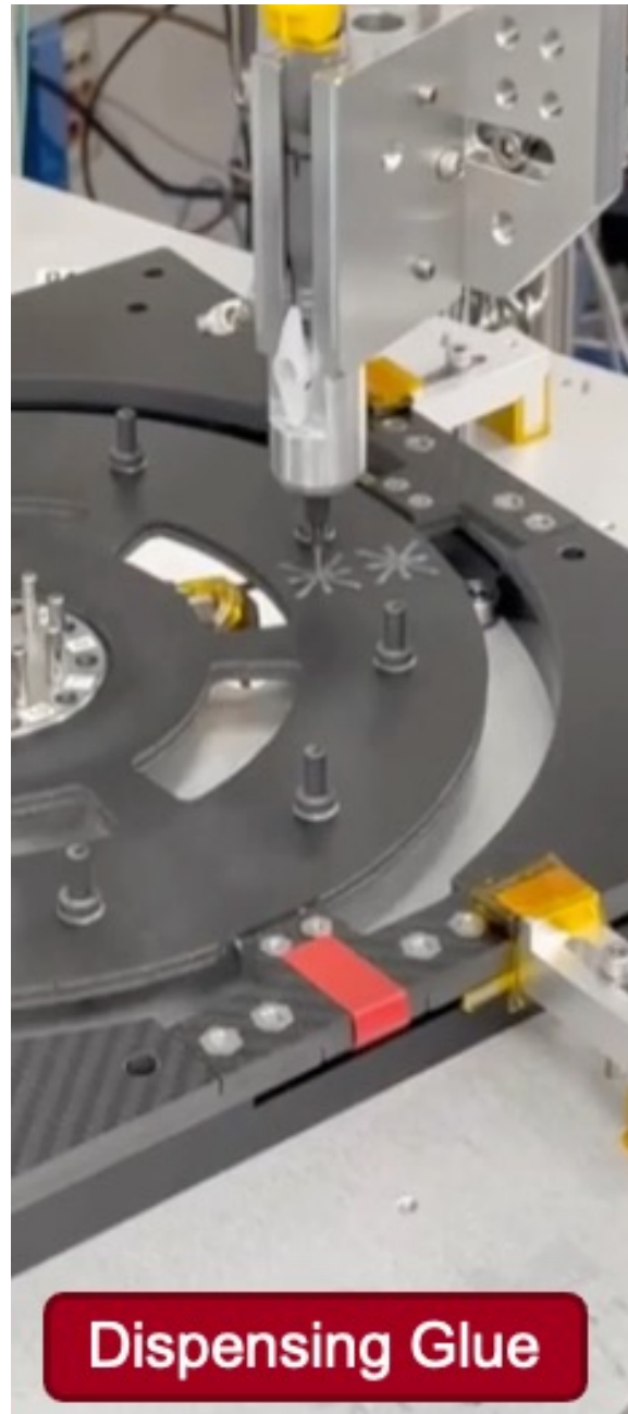
Figure 63: Star pattern being dispensed onto local support ring.
