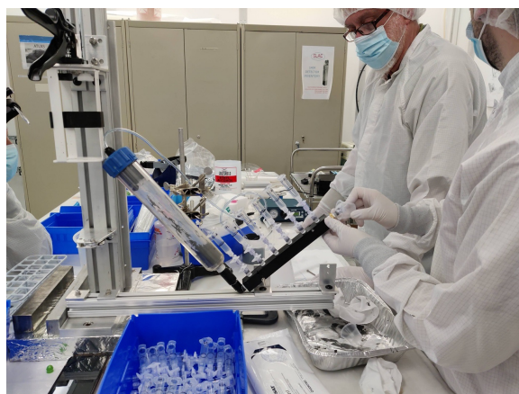
Figure 60: Purging the air out of the manifold prior to pneumatically filling the dispensing syringes.
