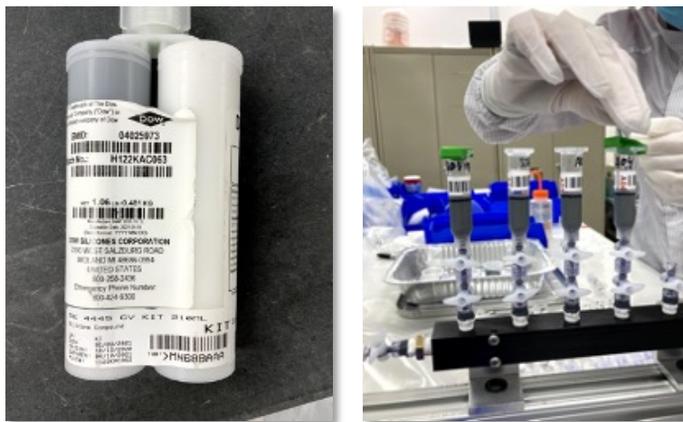
Figure 56: SE4445 as delivered to SLAC, and the filled dispensing syringes.
