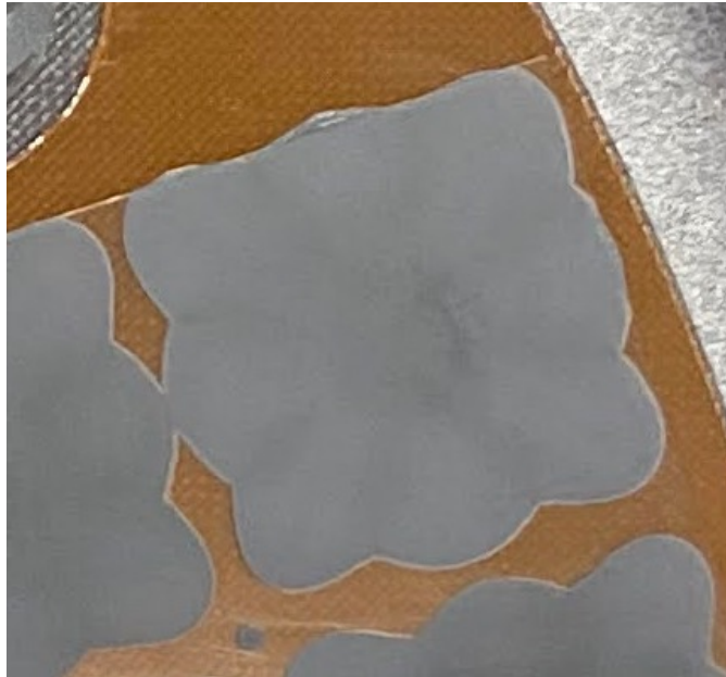
Figure 50: Glue squeeze-out observed when too much glue is dispensed.
