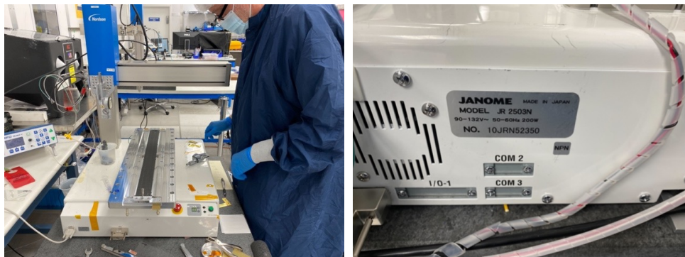
Figure 61: 4D Gantry robot adapted for glue dispensing with stave baseplate loaded.
