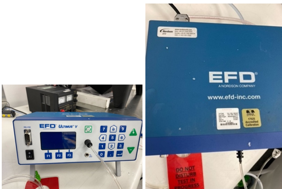
Figure 62: Air actuating pump used for providing back-pressure to dispensing syringes.
