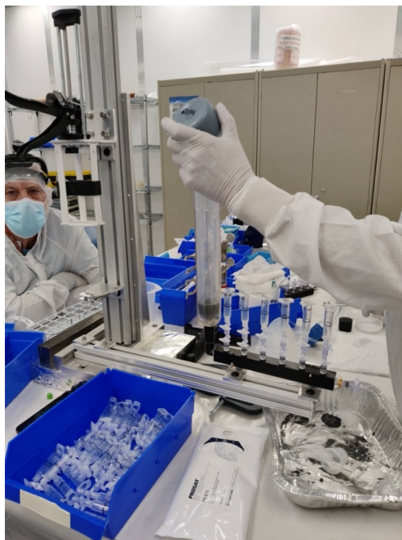
Figure 59: Transferring homogenous glue mixture into large syringe.
