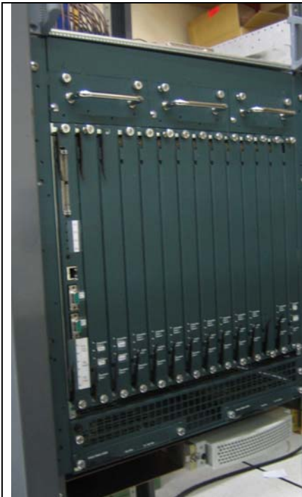
Figure 8.6: Fully occupied Backplane Tester Chassis
