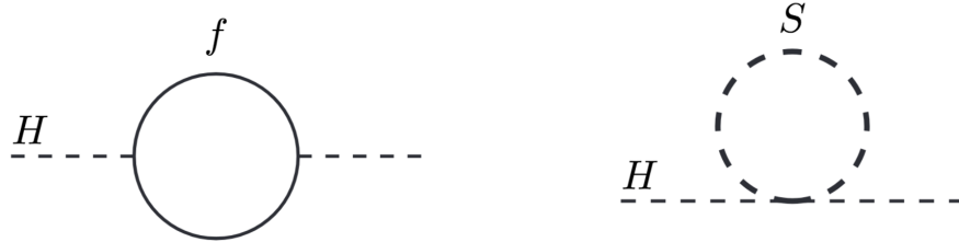
Figure 1.4: One-loop Feynman diagrams for the quantum corrections to the Higgs boson squared mass due to fermions (left) and bosons (right) [29].
