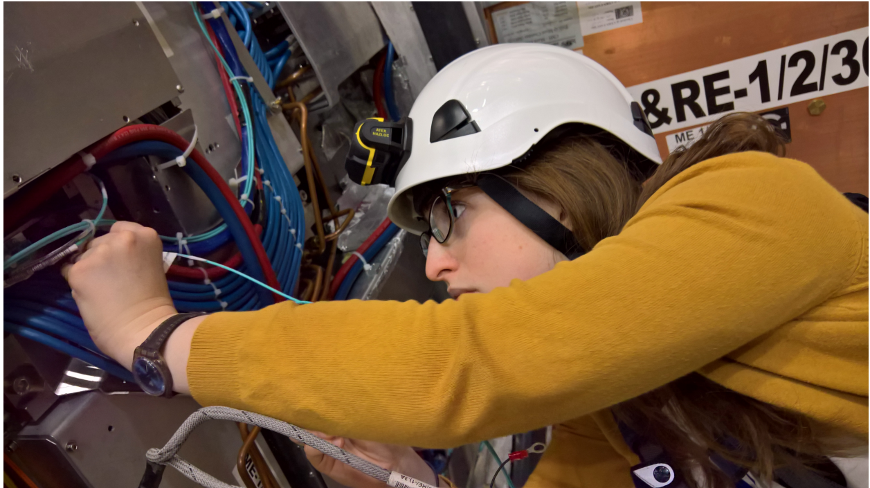
Figure A.2.6: Connecting trigger fibers between CSC and GEM chambers.
