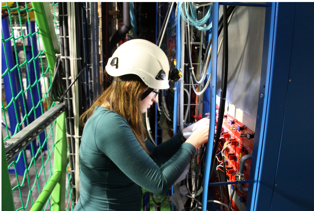
Figure A.2.5: Connecting the low voltage power supply.
