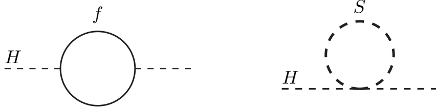
Figure 3.1: One-loop diagrams that give corrections to the Higgs-boson mass parameter m_H^2 from a fermion f (left) and a scalar S (right) Reprinted from Fig. 1.1 of [20].
